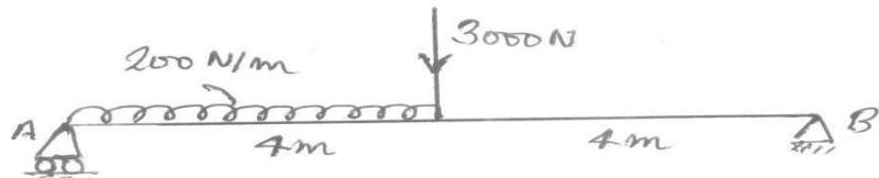
7. A loaded beam shown below, draw its SF and BM diagram.
